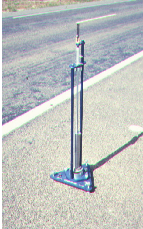
Figure 3: Type 2 ball penetrometer
