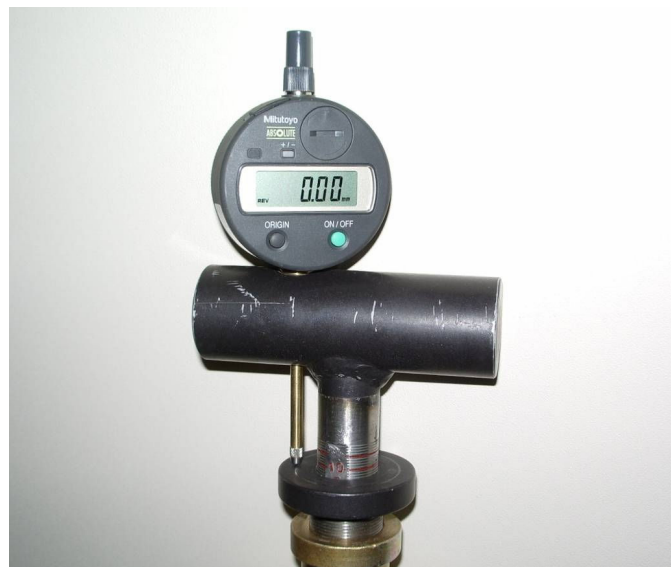
Figure 2: Scribed shaft and optional dial gauge (digital version shown here)
